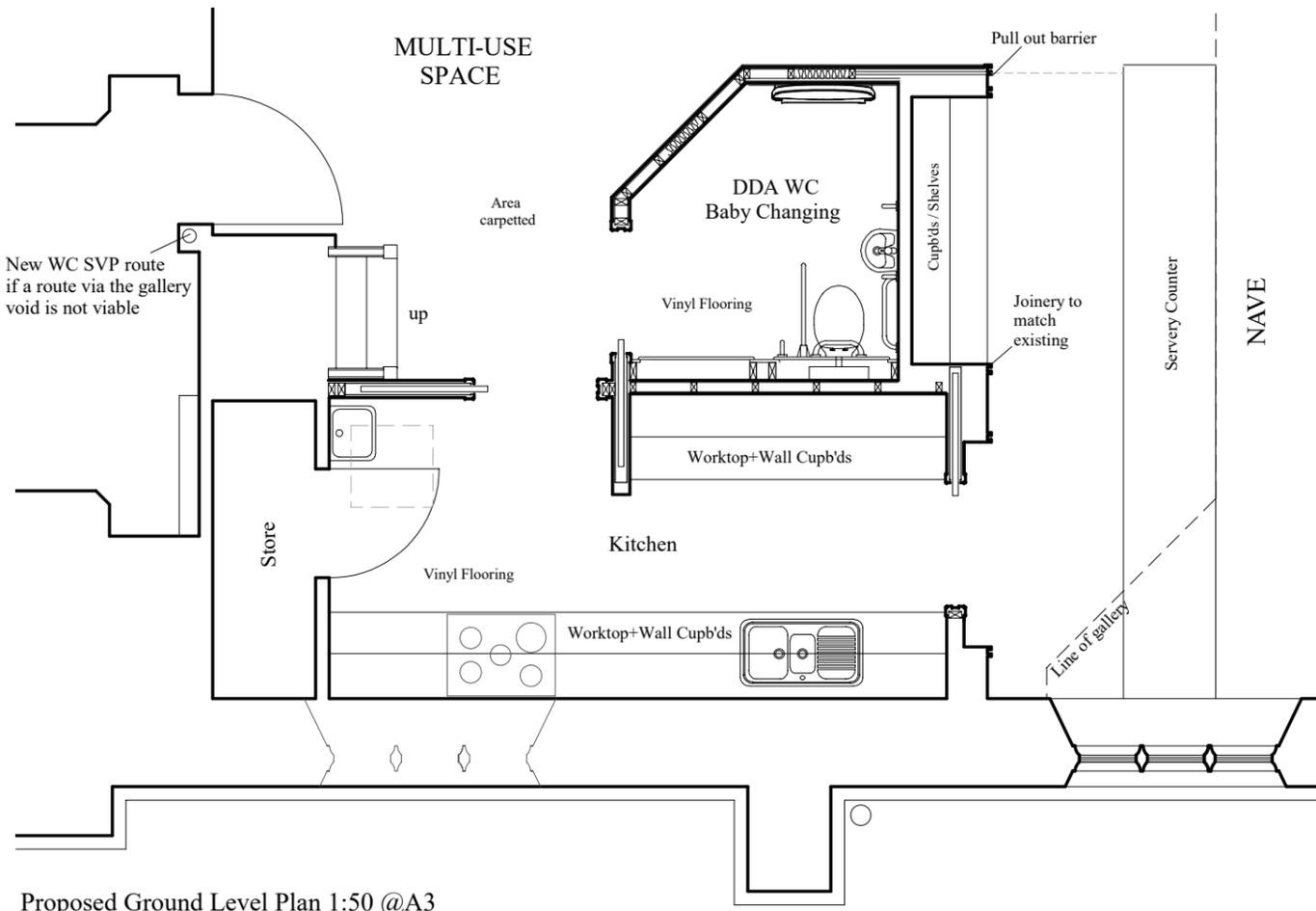
Proposed Ground Level Plan 1:50 @A3
